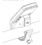
2. Connect the display to the EB-BUS cable.
